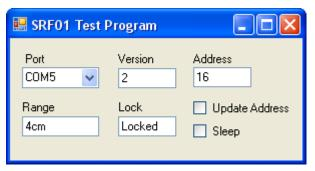
We have a small test program, written in C# which controls the SRF01 via the <u>Acroname S22 or S27</u> modules. A small schottky diode is used to prevent the SRF01 trying to drive the S22/S27's output line (data from the PC). You will need to download and install the <u>FTDI VCP</u> drivers to use the S22/S27.
