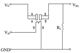
The above is basic test circuit of the sensor. The sensor need to be put 2 voltage, heater voltage(VH) and test voltage(VC). VH used to supply certified working temperature to the sensor, while VC used to detect voltage (VRL) on load resistance (RL) whom is in series with sensor. The sensor has light polarity, Vc need DC power. VC and VH could use same power
