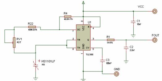
Note: R22=499k $\Omega$  / R4=49.9k $\Omega$  / R1=1 k $\Omega$  / RV1=50 k $\Omega$  potentiometer / C1=10nF / C2=2.2nF / C3=100nF
