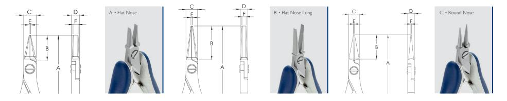
A. - B. flat nose pliers feature a very fine tip, smooth or serrated jaws and inner edges C. round nose pliers have jaws formed by two cones. A round nose pliers is generally used both to clamp and to form loops on leads or wire.
