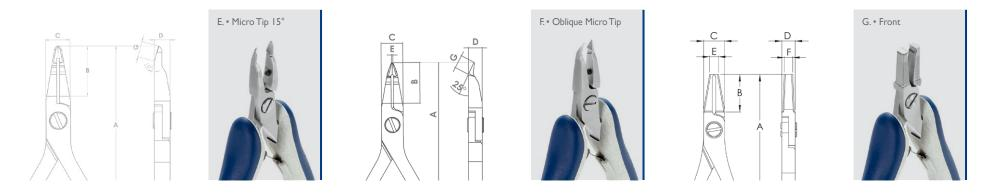
E. - F. long, narrow jaws. Sharp edges for cutting at the very tip. Deep relief for an exceptionally low profile G. tip cutters for vertical tip cutting
