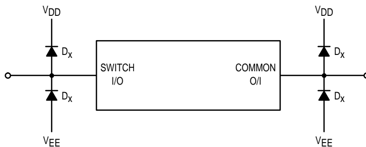
Figure B. External Schottky or Germanium Clipping Diodes
