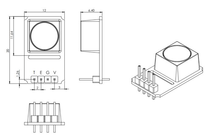
• Connector: 2.0 mm pin header 4 pin
